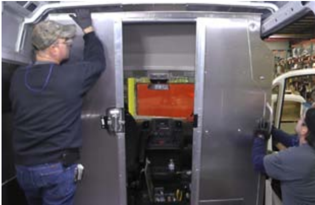
Position bulkhead in cargo area
